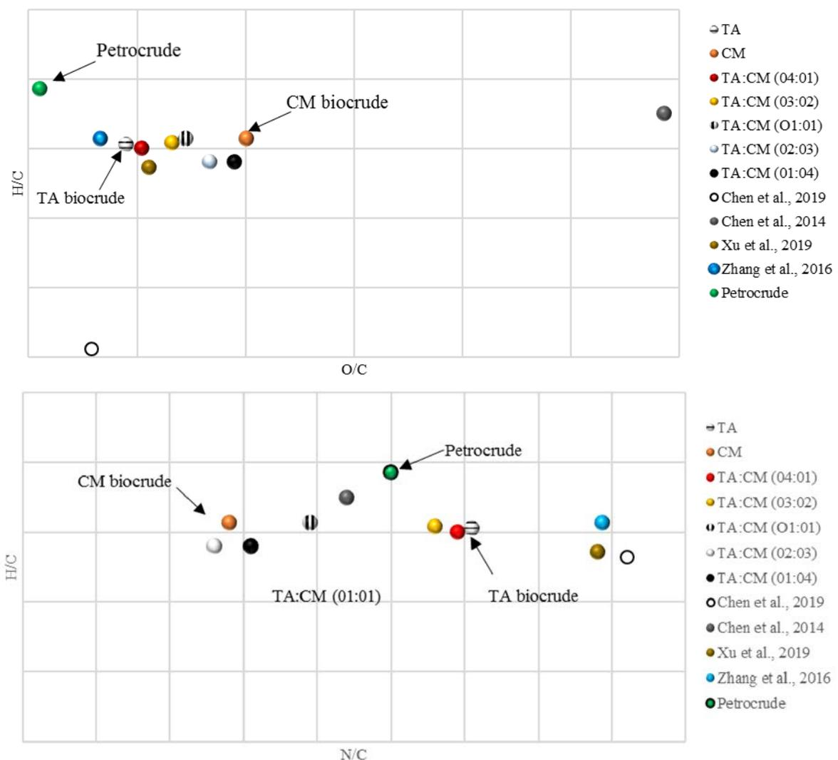
**Fig.3: Van Krevelen diagram showing atomic ratios after co-liquefaction at 350°C.**
