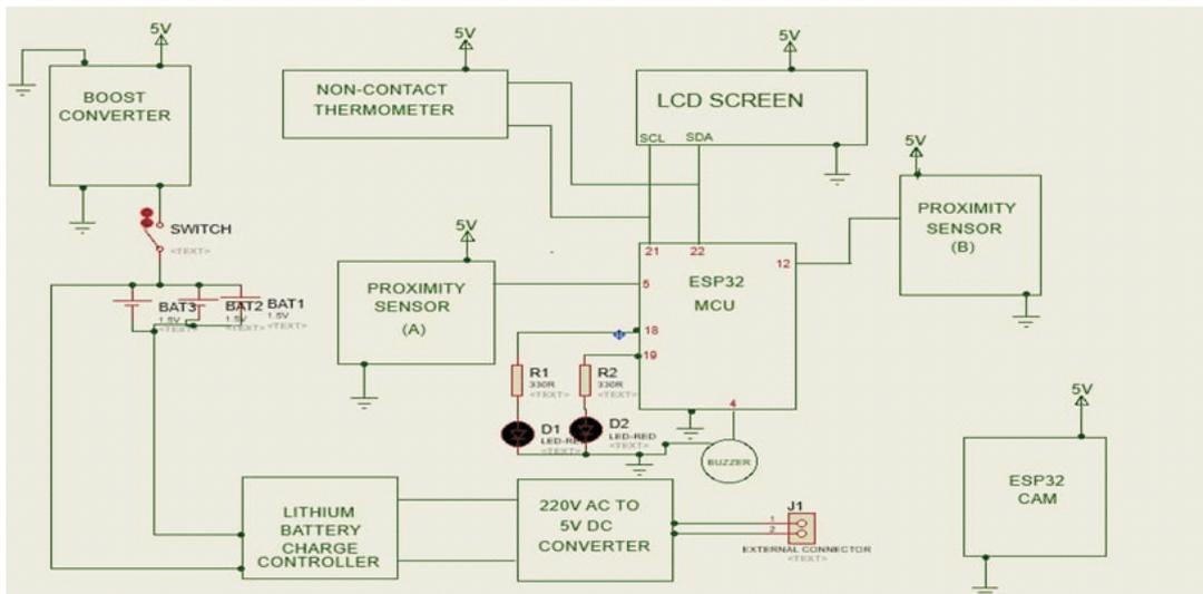
Figure 1: Circuit diagram of the proposed System
