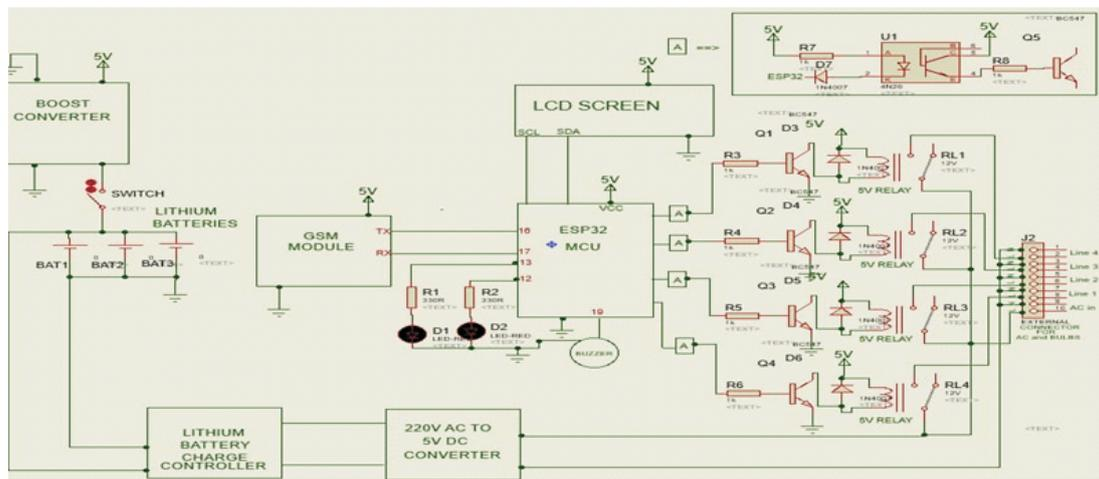
Figure 2: Circuit Diagram of the various modules of the Micro-Controller unit
