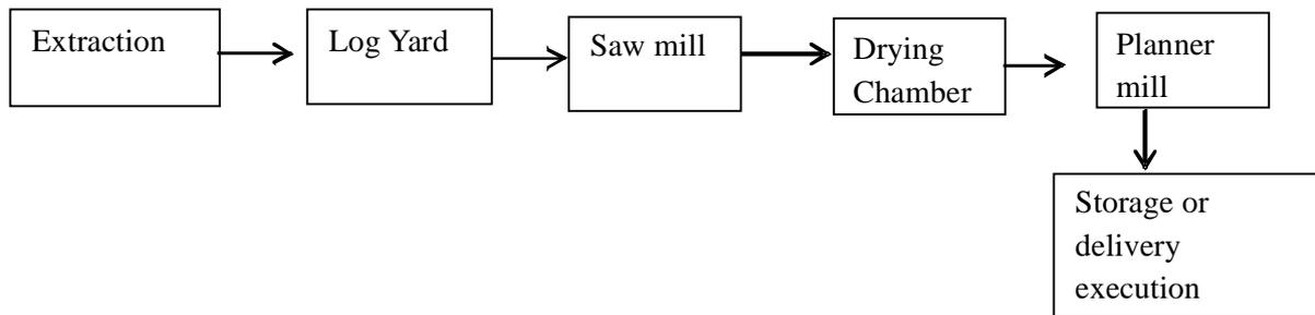
**Figure 1: Unit operations of a Typical timber saw mill (Ohagwu and Ugwuishiwu, 2011).**
