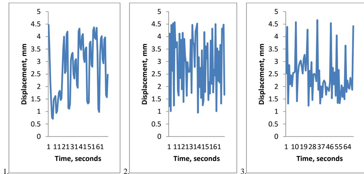
**Figure 13** Displacement time of the mechanical vibration at low frequency (1 – 5 Hz) and low amplitude (5 mm)
