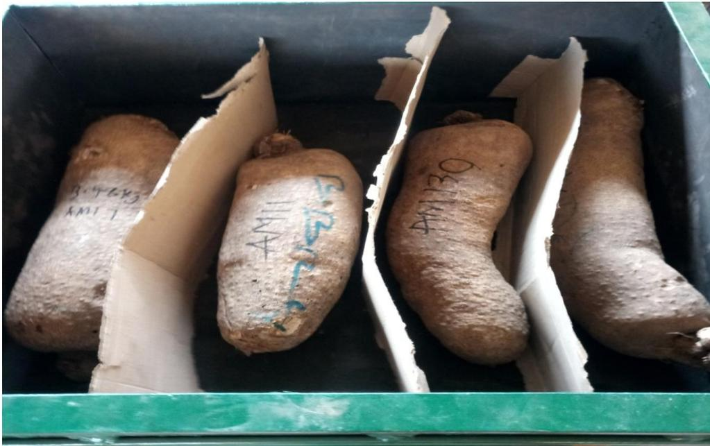
**Plate 3** The view showing the alignment of the yam tubers (weight between 0.1 kg and 2.9 kg and weight 3.0 kg and 5.0 kg) during the vibration
