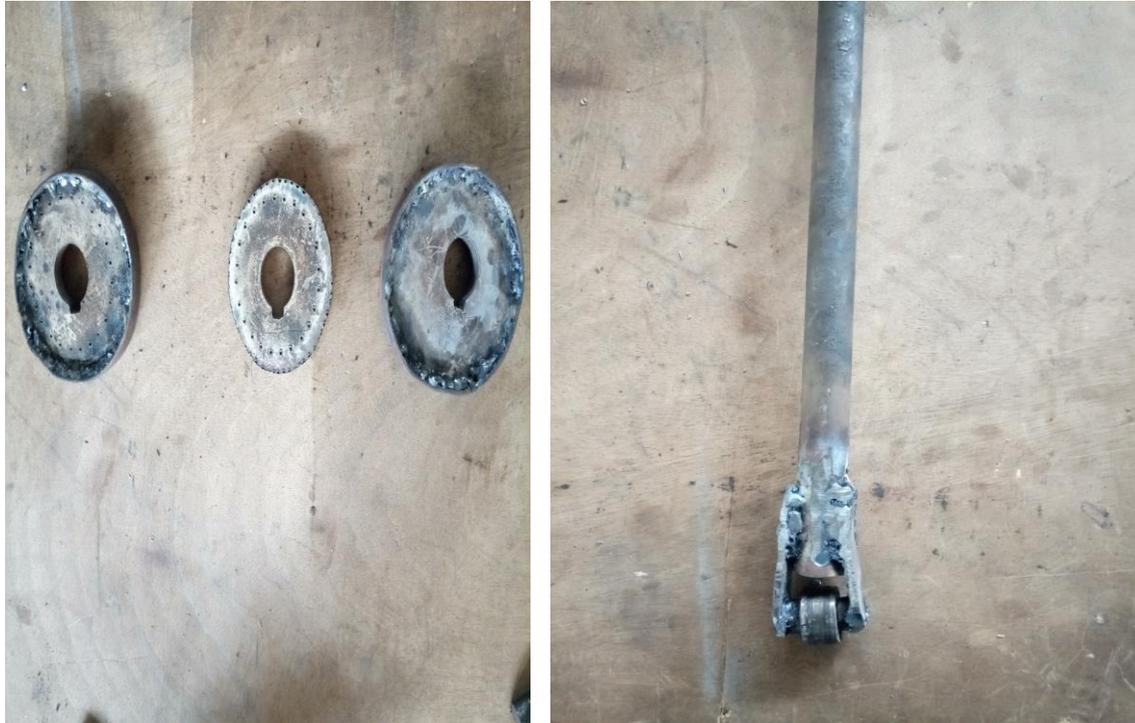
**Plate 1** The view of the 10 mm, 5 mm and 20 mm amplitude (maximum displacement) cycloid cam respectively of the mechanical yam vibrator
