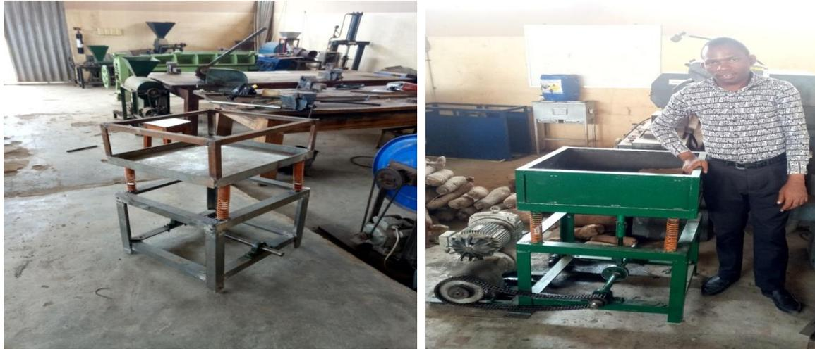
**Plate 1** View of the mechanical yam vibrator during construction
