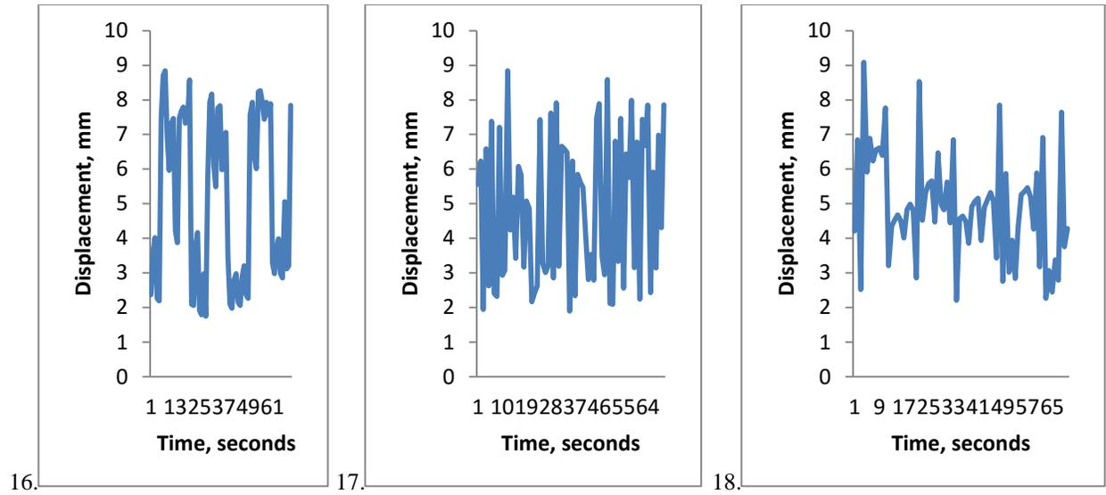
**Figure 16.** Displacement time of the vibration at low frequency (1 – 5 Hz) and medium amplitude (10 mm)
