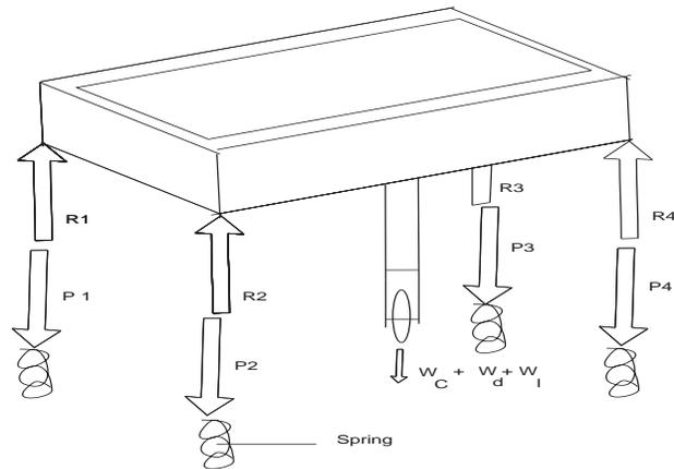
**Figure 7** Freebody diagram of the vibrating chamber and the spring
