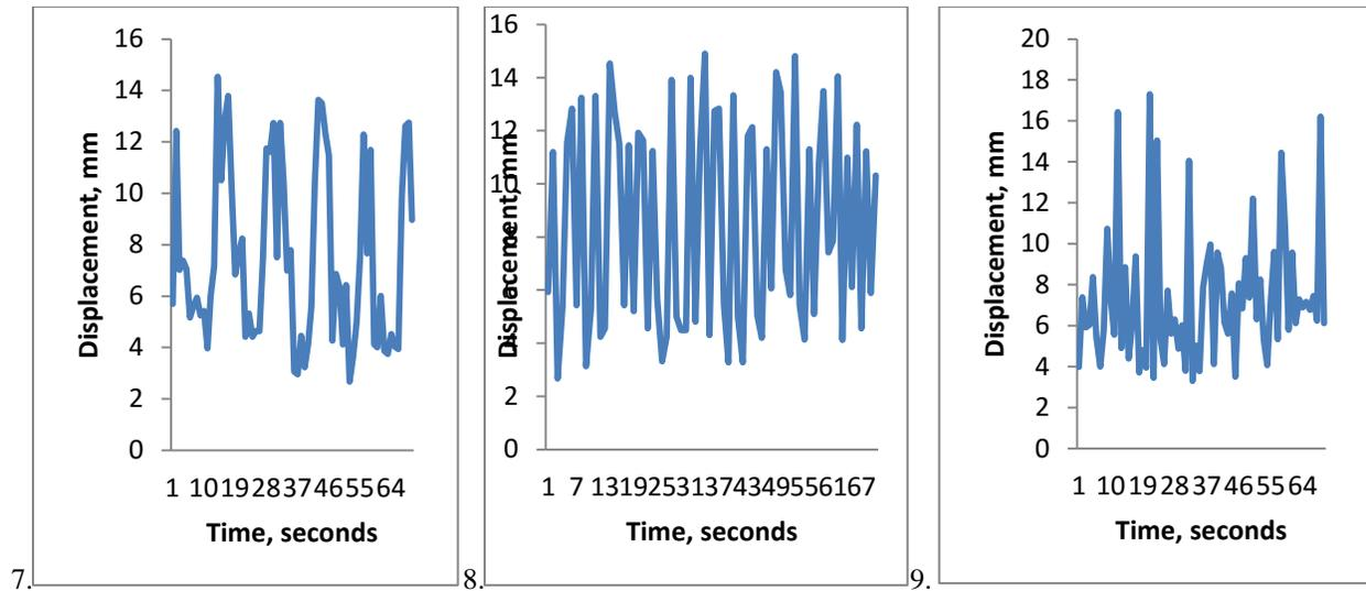
**Figure 19.** Displacement time of the mechanical vibration at low frequency (1 – 5 Hz) and high amplitude (20 mm)
