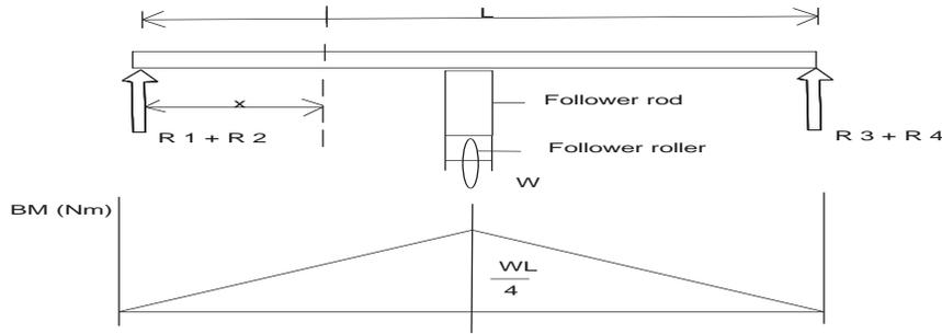
**Figure 4** The bending moment diagram of the vibration chamber
