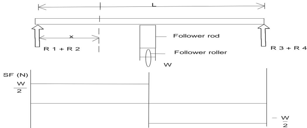
**Figure 6** Shearing force diagram of the vibrating chamber
