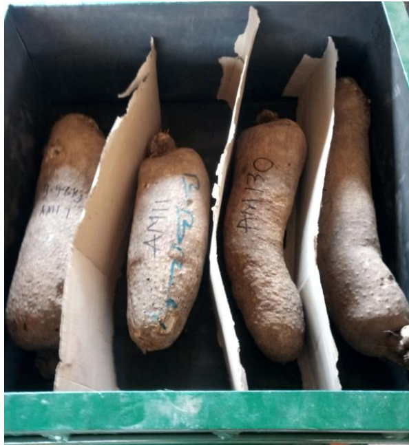
Plate 2: The view showing the alignment of the yam tubers (weight between 0.1 kg and 2.9 kg and weight 3.0 kg and 5.0 kg) during the vibration
