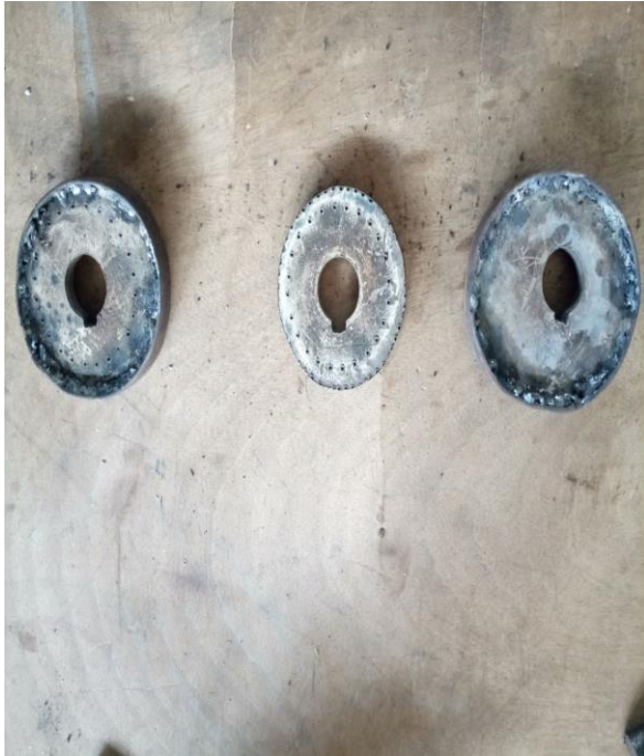
Plate 1: (A) The view of the 10 mm, 5 mm and 20 mm amplitude (maximum displacement) cycloid cam respectively of the mechanical yam vibrator (B) The view of the roller and follower of the mechanical yam vibrator.
