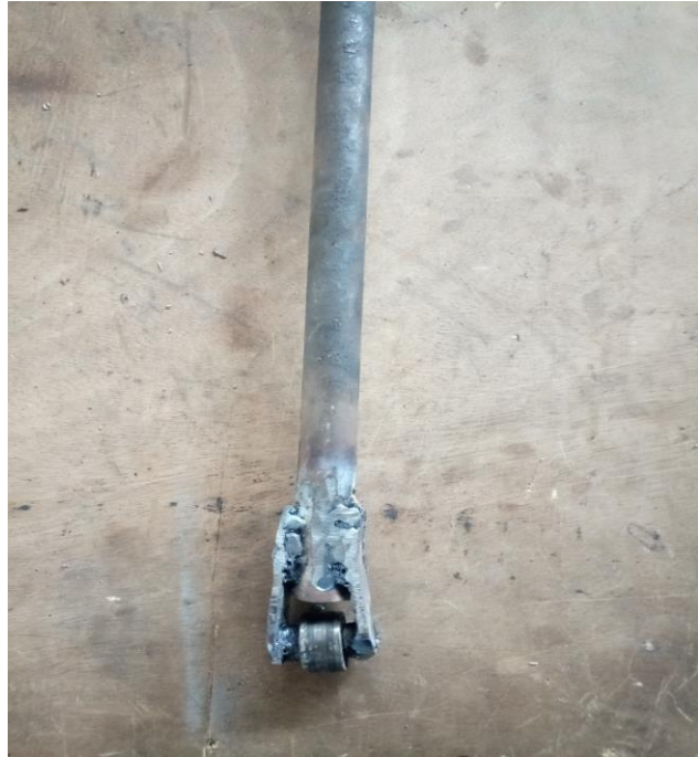
Plate 1: (A) The view of the 10 mm, 5 mm and 20 mm amplitude (maximum displacement) cycloid cam respectively of the mechanical yam vibrator (B) The view of the roller and follower of the mechanical yam vibrator.
