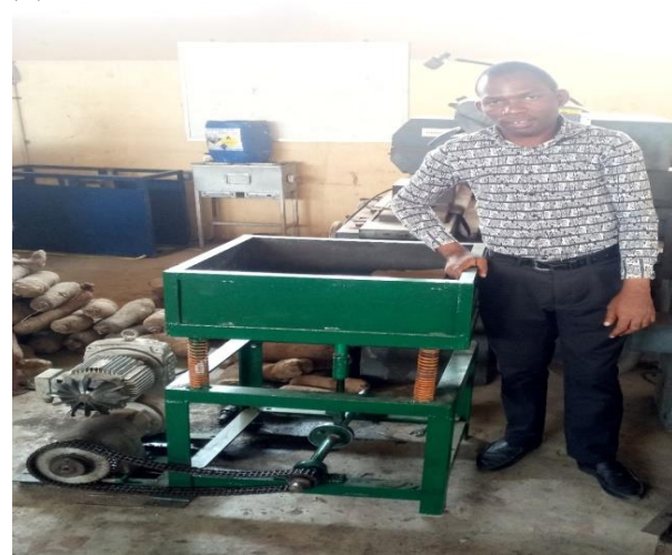
Plate 3: (A) View of the mechanical yam vibrator during construction (B) The view of the developed mechanical yam vibrator with adjustable frequency and amplitude.
