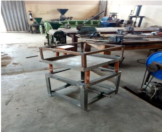
Plate 3: (A) View of the mechanical yam vibrator during construction (B) The view of the developed mechanical yam vibrator with adjustable frequency and amplitude.
